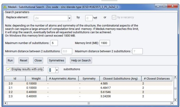
To start with, select which element to replace (here: Zn) and select an element to replace by (here: vacancy). You can use additional parameters to limit the search, e.g. by defining a minimal or maximal distance between two substitutions.
