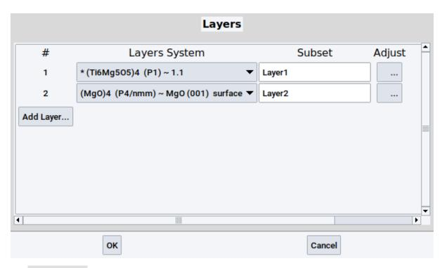
The Layer System: specifies the system to be used to create individual layers. Clicking on this entry displays a list of eligible P1 models.
