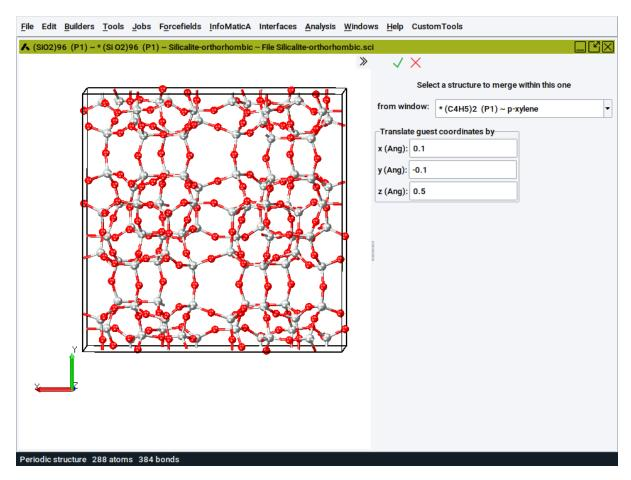
If the two models don't share the same lattice vectors, you can shift the second system in the bigger first system, as defined by a translation vector. Please take care that the second system has smaller or equal dimensions than the first model.
