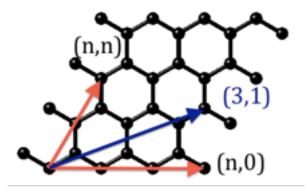
Type of nanotube: Nanotubes are defined by a chirality vector (n,m) which corresponds to how you fold a sheet of graphene into a tube. The two simplest nanotube orientations are armchair (n,n), and zigzag (n,0) and the corresponding chirality vector is shown in red.
