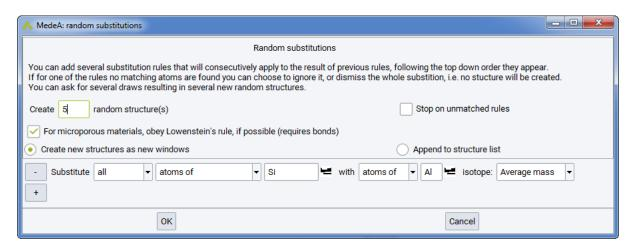
Use Random substitutions... to replace atoms and atomic masses in the current model. Any existing symmetry is reduced to P1.
