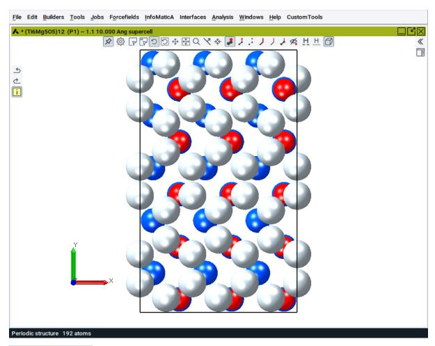
Split in two surfaces: Lets you split the interface into the two corresponding subsystems (surfaces). Use this option when calculating, e.g., the work of separation for an interface.
