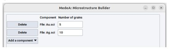
Add component: Add a component to the list of components. This can be either imported from a .sci file or from a model window in *MedeA*. The structure needs to be periodic. For every component the number of grains needs to be set as a positive integer. The default number of grains is 5.
