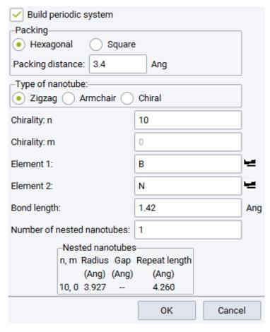
Packing: You can select *hexagonal* or *cubic* packing in the plane normal to the nanotube direction. The distance between nanotubes is defined by *Packing distance* (in Angstrom).
