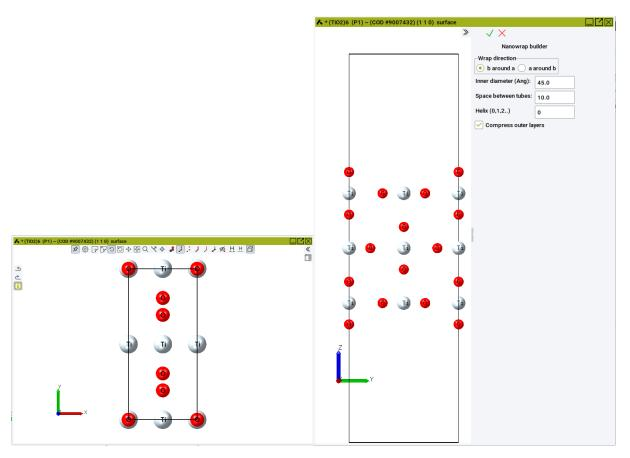
The top surface is going to be inside of a tube, the bottom surface outside. You have (at least) two choices to wrap a\_around\_b or b\_around\_a. To create the desired structue click on the tick icon  $\checkmark$ .
