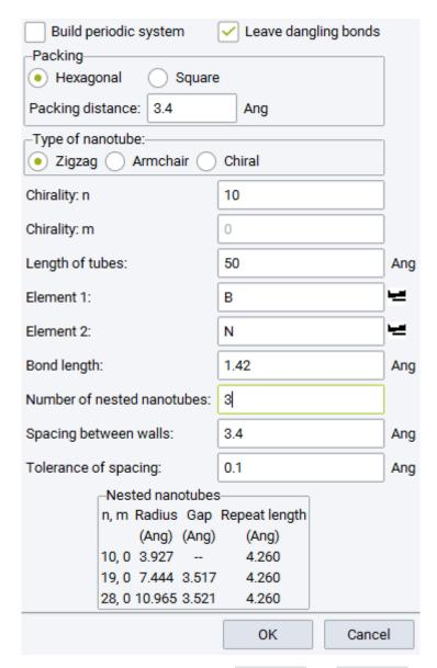
You can easily create nanotubes of B-N by changing the Element 1, the Element 2, and the Bond length.
