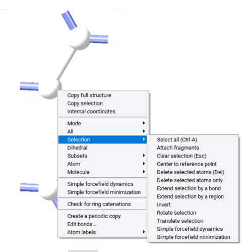
Dihedral appears as entry below Selection. Displays dialog to view and edit the dihedral angle including the choice which of the two atoms at the end of the chain to displace when changing the angle. This option requires 4 linearly bonded atoms.
