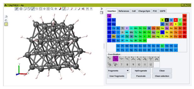
In the illustration below a spherical Ag nanoparticle with 10  $\rm \mathring{A}$  diameter is passivated with hydrogen (with one-fold coordination).
