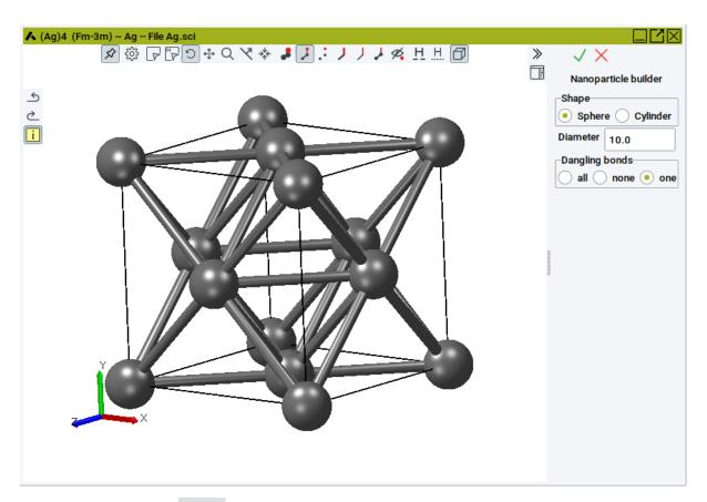
You need to specify the shape as a *sphere* or a *cylinder* and set the size by diameter and length (for cylinder). Dangling bonds allow you to keep *all* existing bonds at the boundary or only *one* (for passivation) or *none*.
